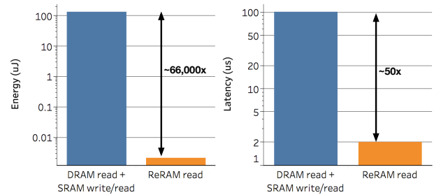
Figure 11: Costs of reading all embedding weights after system power-on. Storing embeddings in ReRAMs gives EdgeBERT significant energy and latency advantages compared to the conventional approach requiring DRAM read followed by SRAM write/read.
